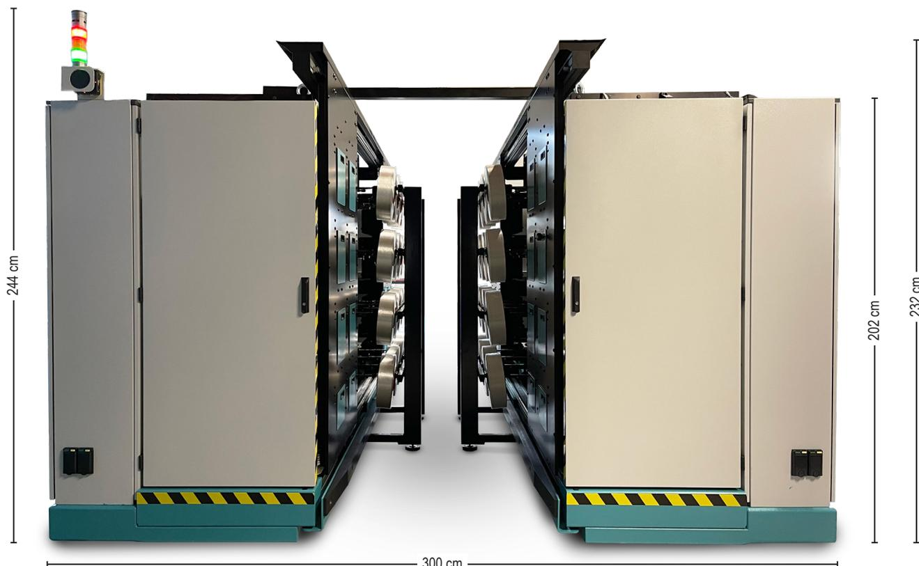
**Ra Vision** was born from the technical expertise of our team combined with our 30 years experience in the textile field, with the goal of providing objective and repetitive results. Ra Vision combines optical systems, electronic boards, mechanical parts and software code to control the quality of your bobbins. All these elements are designed and managed by Thema2.
